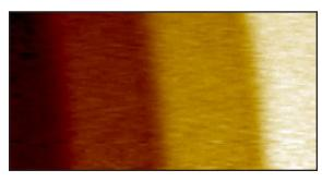
SiC with 1.5nm steps  $1.5\mu m \times 0.75\mu m$  Data taken with QS-PLL<sup>TM</sup> with Nano-3D200 nanopositioning system and tungsten tip on a quartz tuning fork.
